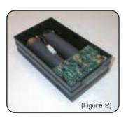
MLBATT-PSM2: (Figure 2) A PSM is incorporated into the standard ModuLogger/Mini ML-BATT module (six D-cell plug-on battery pack). A terminal strip provides for easy connection/disconnection of the control, external power, and output voltages.
