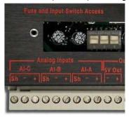
Only the first two of these Channels (AI\_A and AI\_B) can be configured as Thermocouples. The Thermocouple icon performs the thermocouple channel selection, amplification, CJC and A-D conversion for thermocouple hardware Input. The CJC reading is taken from the thermal sensor on the CPU, described above.
