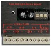
The CPU has three channels that can be configured this way. The last of these Channels (AI\_C) has a fixed gain, so when it is configured as a Current icon it is limited to the range 0.0 to +32 mA. The mA Input icon performs the analog channel selection, amplification, and A-D conversion for a DC current Input within the range of -12 to +20 mADC.
