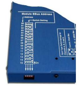
Note: Address zero is reserved. It must not be used on the BBus.
