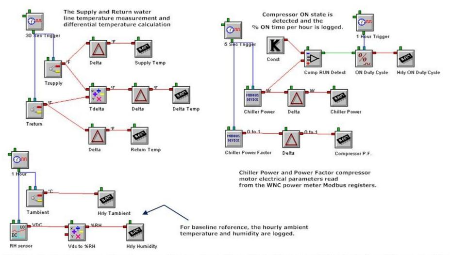
Chiller Temperatures, Compressor Power, Run-Time Duty-Cycle and Ambient Condition Logging
