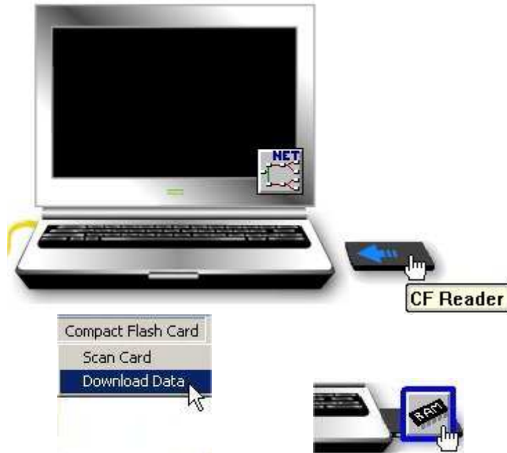
Figure 8-2; Downloading Data from a CF Card
